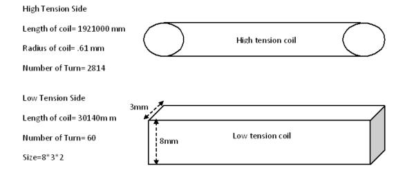
Figure: Internal Data of 100 KVA Transformer
