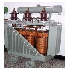
Cut-away view of three-phase oil-cooled transformer. The oil reservoir is visible at the top. Radiative fins aid the dissipation of heat.
