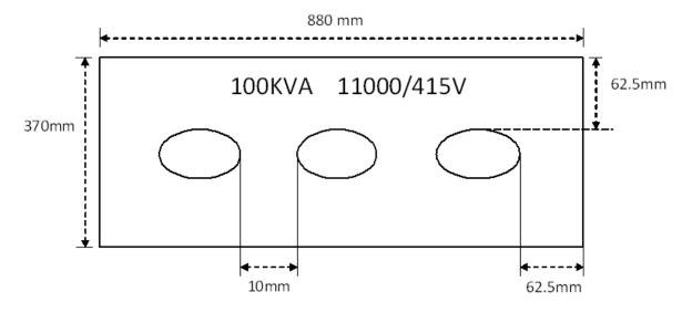
Figure: Side view of a transformer
